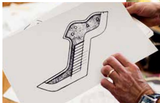
1990 Hytrel thermoplastic collar lockdown strap sketch
